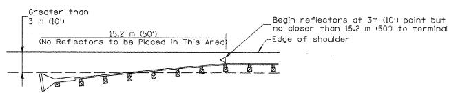
NOTE: Omit terminal marker when terminal over (10') from edge of paved shoulder or break point of unpaved shoulder.
