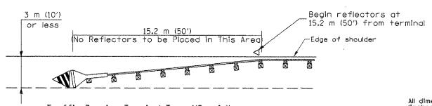
Traffic Barrier Terminal Type 1(Specia) [Terminal 3 m (10') or less from edge of shoulder] All dimensions are in millimeters (inches) unless otherwise noted.
