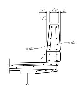
EXISTING SECTION THRU PARAPET
