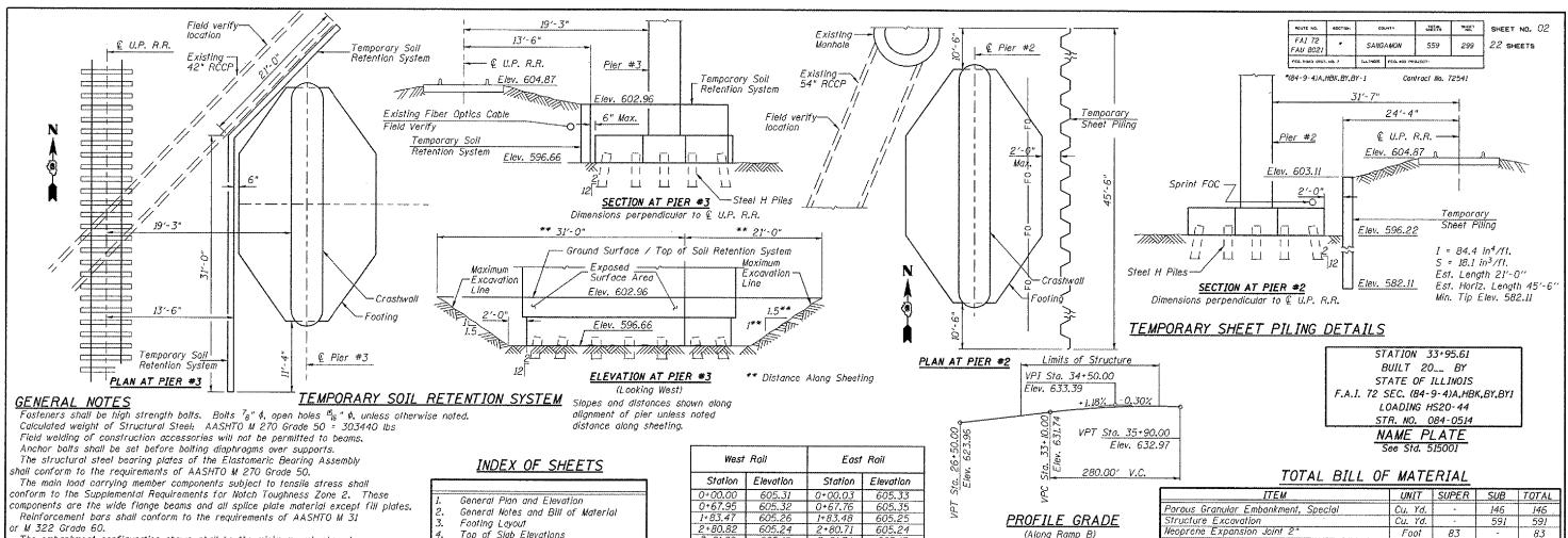
The embankment configuration shown shall be the minimum embankment that must be constructed prior to construction of the abutments.
