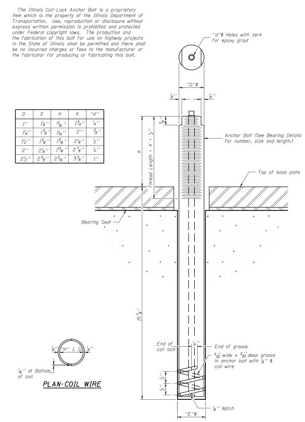
ILLINOIS COIL-LOCK ANCHOR BOLT
