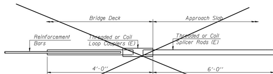
**FOR INTEGRAL OR SEMI-INTEGRAL ABUTMENTS**
