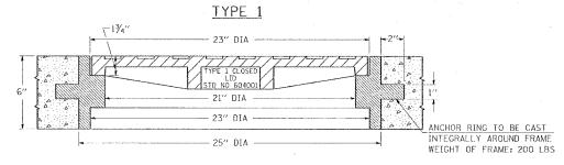
THE FRAMES MAY BE MADE OF EITHER GRAY IRON CONFORMING TO THE STANDARD SPECIFICATIONS OR DUCTILE IRON CONFORMING TO THE SPECIFICATIONS FOR DUCTILE IRON CASTING, A.S.T.M. DESIGNATION:
