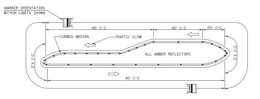
$\begin{array}{c} \underline{\text{NOTES}} & \text{1. PRISMATIC REFLECTORS SHALL BE MONO-DIRECTIONAL AND POSITIONED} \\ & \text{SO THAT THE REFLECTIVE FACE IS FACING THE APPROACHING TRAFFIC.} \end{array}$
