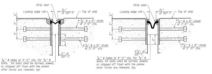
SECTION THRU ROLLED RAIL JOINT
