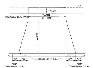
ASPHALT DRIVE - 3" BIT. CONC. SURF. COURSE, SUPERPAVE, MIX "C", N50 (QC/QA) 6" AGGREGATE BASE COURSE, TYPE B
