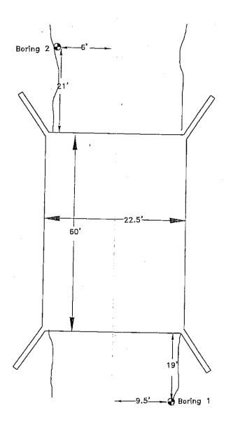
Note: Center of Existing Bridge Elevation = 543.3
