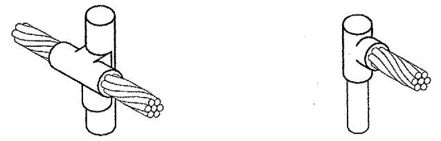
CABLE TO GROUND ROD
