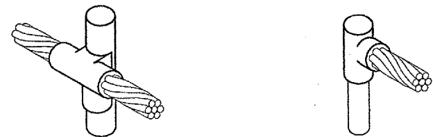
CABLE TO GROUND ROD
