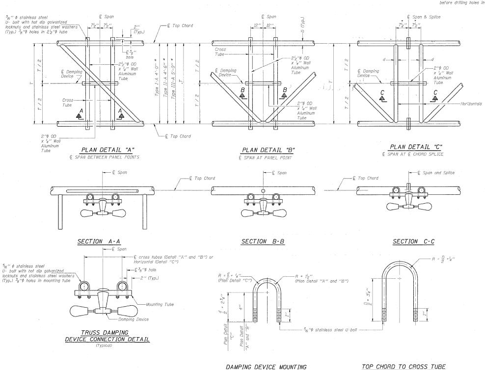
TUBE U-BOLT DETAIL (Typical)
