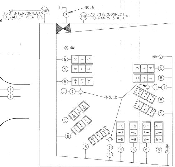
"C" DENOTES COAXIAL AND OTHER NECESSARY CABLES FOR VIDEO DETECTION "G" DENOTES IC NO.6 GROUNDING CABLE TO CONNECT ALL MAST ARMS AND THE CONTROLLER TO THE GROUNDING ROD IN THE DOUBLE HANDHOLE
