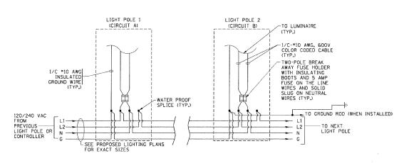
LIGHT POLE WIRING DETAIL
