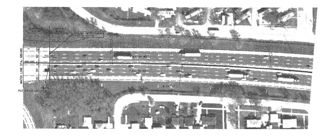
HMA PATCH \* PROPOSED HOT MIX ASPHALT PAVEMENT PATCH. SEE SCHEDULE OF QUANTITIES
