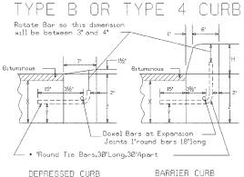
and Combined Curb & Gutter in prolongation with the joints in the pavement. The details of the Transverse Joints in the Curb,Gutter and Combined Curb & Gutter shall be Approved by the COMMISSIONER.Curb,Gutter or Combined shall be corrugated-all Dowel Bars shall be smooth.
