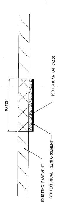
THE CA 6 OR CA 10 SHALL BE COMPACTED IN A MANNER APPROVED BY THE ENGINEER. IF THE MOISTURE CONTENT OF THE MATERIAL IS SUCH THAT COMPACTION SATISFACTORY TO THE ENGINEER CANNOT BE OBTAINED, SUFFICIENT WATER SHALL BE ADDED SO THAT SATISFACTORY COMPACTION SHALL BE ADDED S CAN BE OBTAINED. THE CA 6 OR CA 10 WILL BE PAID FOR AT THE CONTRACT UNIT PRICE PER CU 'YD FOR GRANULAR SUBGRADE REPLACEMENT
