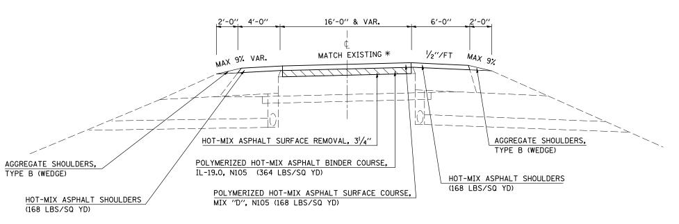
\* SLOPE VARIES IN SUPERELEVATION AREAS WITH A MAXIMUM OF 0.08 FT/FT DIFFERENCE IN PAVEMENT GRADE AND SHOULDER GRADE.
