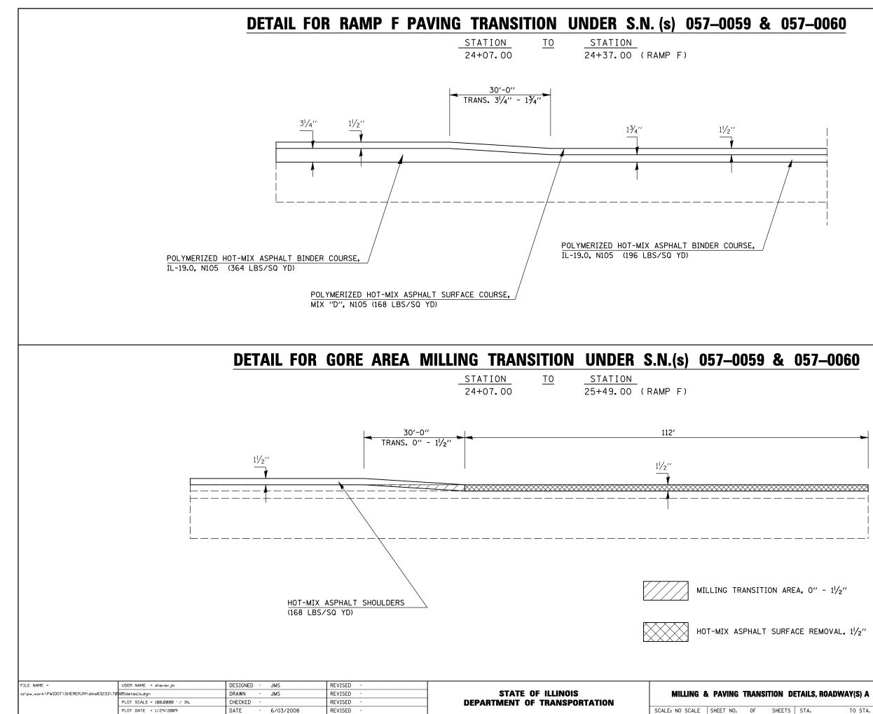
NOTE: AREA OF MILLING TRANSITION SHALL BE INCLUDED IN THE CONTRACT UNIT PRICE FOR THE VARIOUS PAY ITEMS FOR HOT-MIX ASPHALT SURFACE REMOVAL OF THE DEPTH SPECIFIED AND NO ADDITIONAL COMPENSATION SHALL BE ALLOWED.
