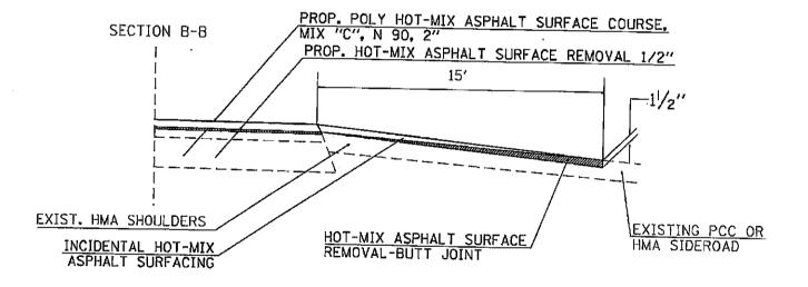
IF EXISTING BASE COURSE IS INADEQUATE, AS DETERMINED BY THE ENGINEER, THE SIDEROADS SHALL BE CORED OUT AND AGGREGATE BASE COURSE, TYPE B SHALL BE PLACED FOR BASE. THE COST OF CORING OUT THE SIDEROAD SHALL BE INCLUDED IN THE COST OF THE AGGREGATE BASE COURSE. IF EXISTING BASE COURSE IS DETERMINED TO BE ADEQUATE, THE AGGREGATE BASE COURSE SHALL BE DELETED AND THE PREPARATION OF THE BASE SHALL BE CONSTRUCTED ACCORDING TO ARTICLE 406.19.
