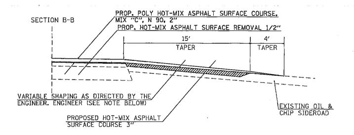
IF EXISTING SUB-BASE IS INADEQUATE, AS DETERMINED BY THE ENGINEER, THE SIDEROADS SHALL BE CORED OUT AND AGGREGATE SUB-BASE, TYPE B SHALL BE PLACED FOR BASE. THE COST OF CORING OUT THE SIDEROAD SHALL BE INCLUDED IN THE COST OF THE AGGREGATE BASE COURSE. IF EXISTING SUB-BASE IS DETERMINED TO BE ADEQUATE, THE AGGREGATE BASE COURSE SHALL BE DELETED AND THE PREPARATION OF THE BASE SHALL BE CONSTRUCTED ACCORDING TO ARTICLE 406.19 VARIABLE SHAPING IS INCLUDED IN THE COST OF BITUMINOUS CONCRETE.
