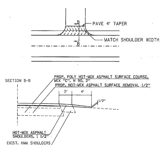
PREPARATION OF EXISTING SURFACE AND ANY EXCAVATION FOR ENTRANCES SHALL BE IN ACCORDANCE WITH ARTICLE 406.19 OF THE STANDARD OF SPECIFICATIONS.
