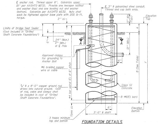
Provide conduit openings both poles. .
