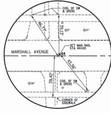
BASELINE TIE STATION 44+00.00
