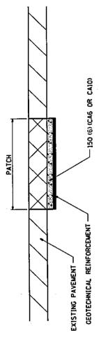
THE CA 6 OR CA 10 SHALL BE COMPACTED IN A MANNER APPROVED BY THE ENGINEER. IF THE MOISTURE CONTENT OF THE MATERIAL IS SUCH THAT COMPACTION SATISFACTORY STATE ENGINEER CANNOT BE OBTAINED, SUFFICIENT WATER SHALL BE ADDED SO THAT SATISFACTORY COMPACTION CAN BE OBTAINED.
