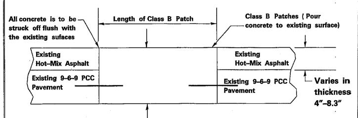
PATCH THICKNESS VARIES -(9" plus thickness of Hot-Mix Asphalt Overlay)
