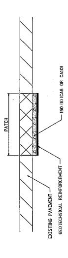
THE CA 6 OR CA 10 SHALL BE COMPACTED IN A MANNER APPROVED BY THE ENGINEER. IF THE MOISTURE CONTENT OF THE MATERIAL IS SUCH THAT COMPACTION SATISFACTORY TO THE ENGINEER CANNOT BE OBTAINED, SUFFICIENT WATER SHALL BE ADDED SO THAT SATISFACTORY COMPACTION CAN BE OBTAINED.
