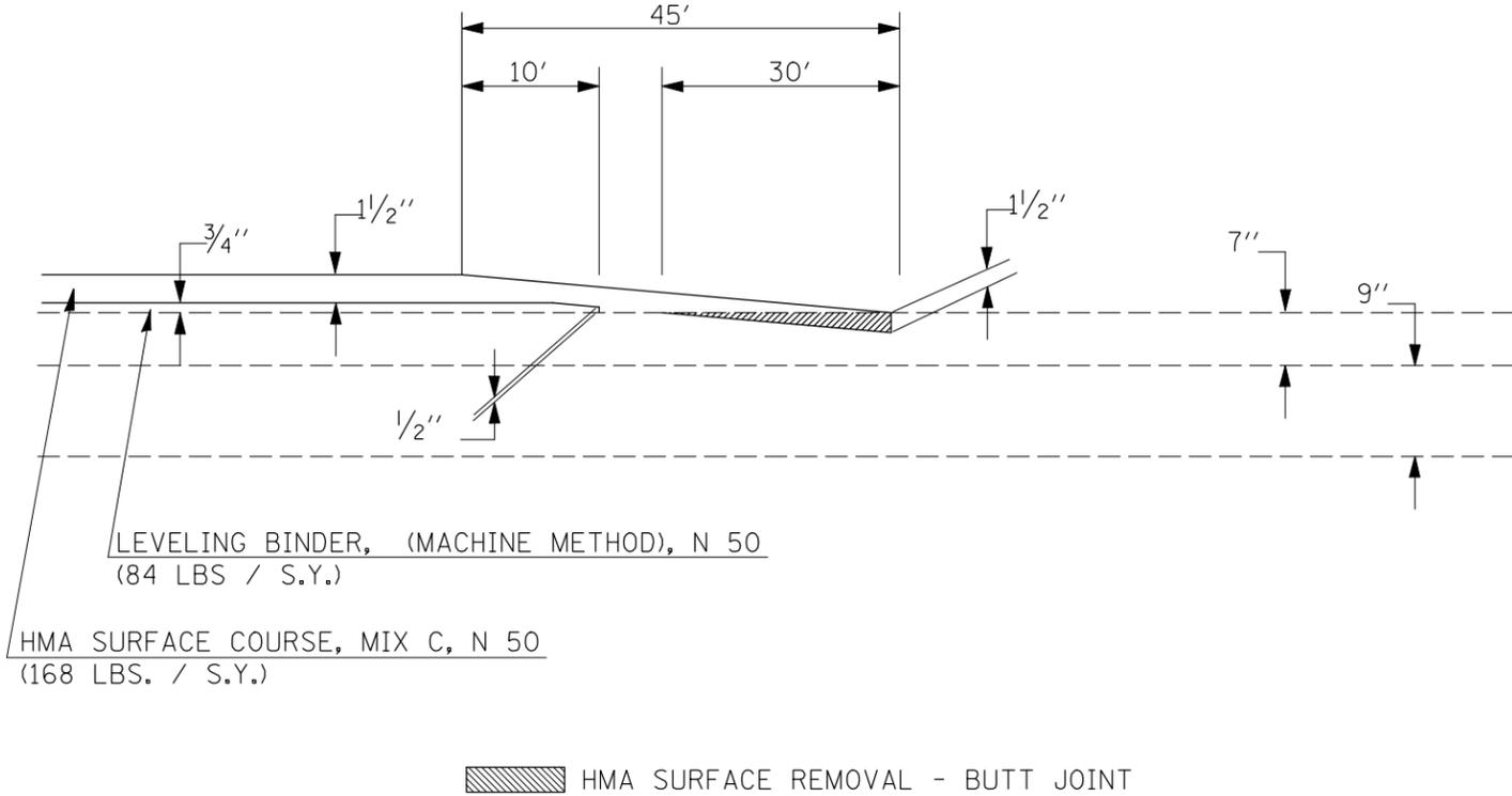
DETAIL OF MILLING TRANSITION FROM 3/4" TO 1/2"
