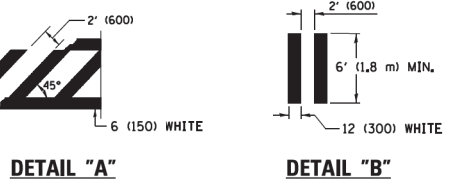
TYPICAL CROSSWALK MARKING
