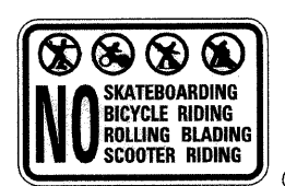
NO SKATEBOARDING SIGN APPROX. 18" X 24" MIN. SHALL BE SIGN PANEL TYPE 1 ON METAL POST TYPE A
