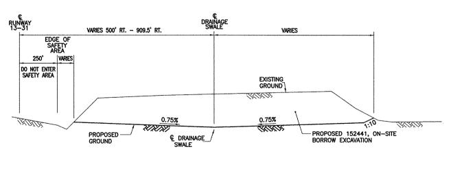
NOTE: SOILS HAULED FROM THE NORTH ON-SITE BORROW AREA TO THE TAXIWAY P CONSTRUCTION SITE AREA SHALL BE PAID FOR BY CUBIC YARDS REMOVED UNDER CONTRACT ITEM 152441, ON-SITE BORROW.
