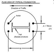
B (Bracket No. 1) = Depth of Post + 202mm (7-15/16") B (Bracket No. 2) = Depth of Post + 205mm (8-1/16")
