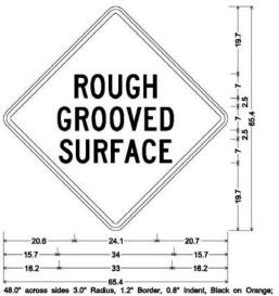
48.0" across sides 3.0" Radius, 1.2" Border, 0.8" Indent, E [ROUGH] C 2K 82% spacing; [GROOVED] C 2K 90% spacing; [SURFACE] C 2K 87% spacing;
