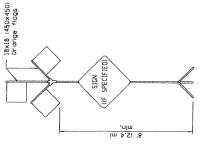
HOAD CONSTRUCTION NEXT X MILES sign shall be placed 500' (150 m) in advance of project limits.
