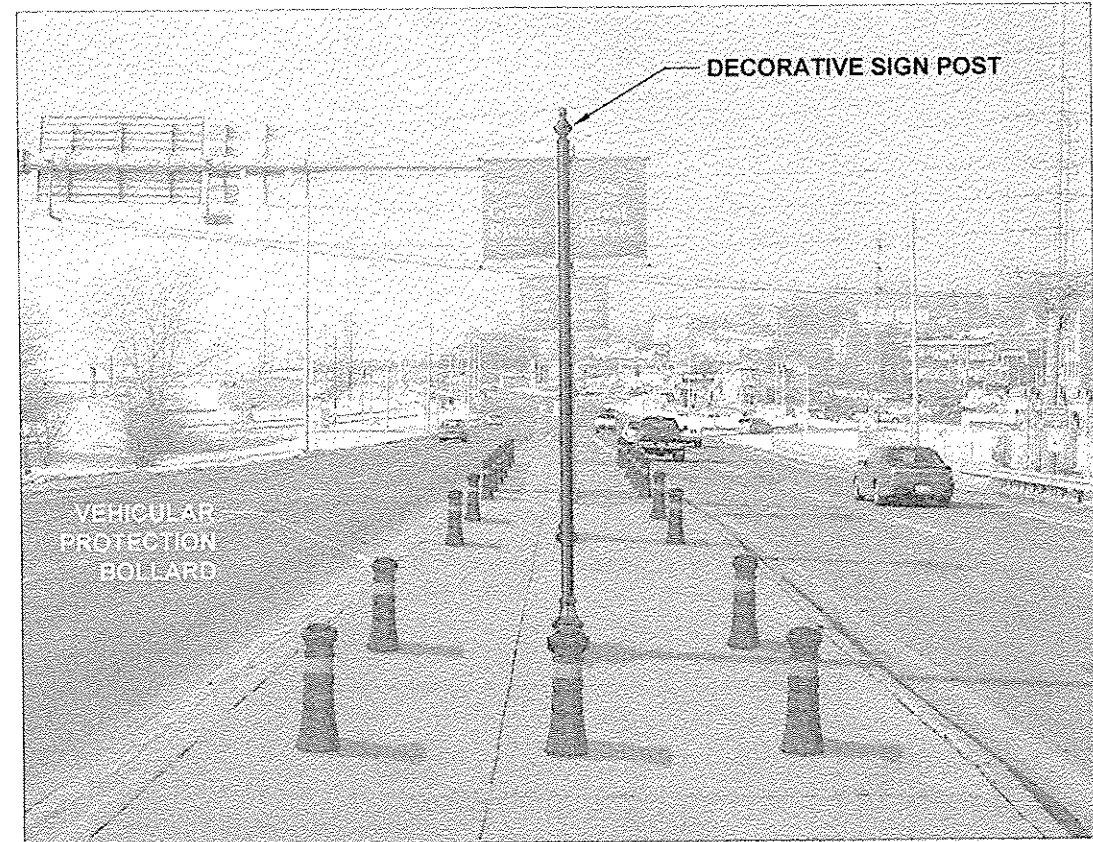
2 46 PLAN MEDIAN LAYOUT PROPOSED IMPROVEMENTS - DECORATIVE SIGN POSTS & VEHICULAR PROTECTION BOLLARDS NTS
