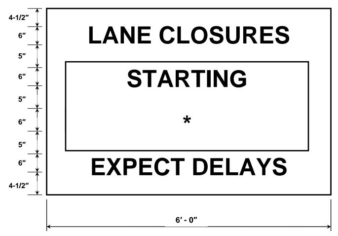
\*Contractor shall provide overlay panel with the date for Start of lane closure. Signs shall be erected a minimum of one (1) week in advance of the start of the work. Overlay panel shall be removed soon after start of construction.
