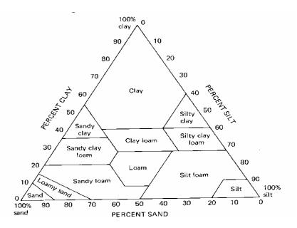
The mechanical analysis should show that the % sand, % silt, and the % clay must yield a silt loam soil. See the attached Textural Classes diagram above. To determine the class plot a line parallel to the % clay axis starting the line at the value of the % silt. Plot another line parallel to the % sand axis starting the line at the value of the % clay. The intersection of these lines should be in the silt loam region, for the soil to be approved.
