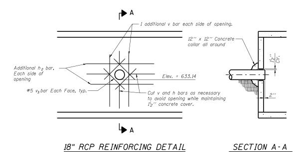
Note: At the Contractor's option delete the concrete collar and cast the wall around the pipe.
