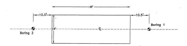
Note: Center of Existing Bridge Assumed Elevation = 100.0
