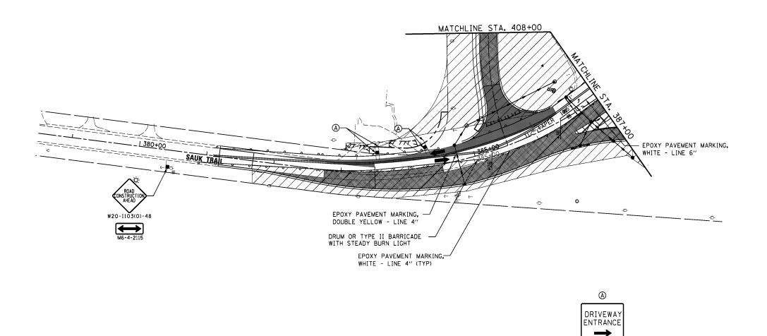
NOTE: FRONTAGE ROAD TO BE BUILT IN SECTIONS TO ALLOW ACCESS TO BUSINESSES. THE FRONTAGE ROAD SHOULD BE COMPLETED IN THIS STAGE.
