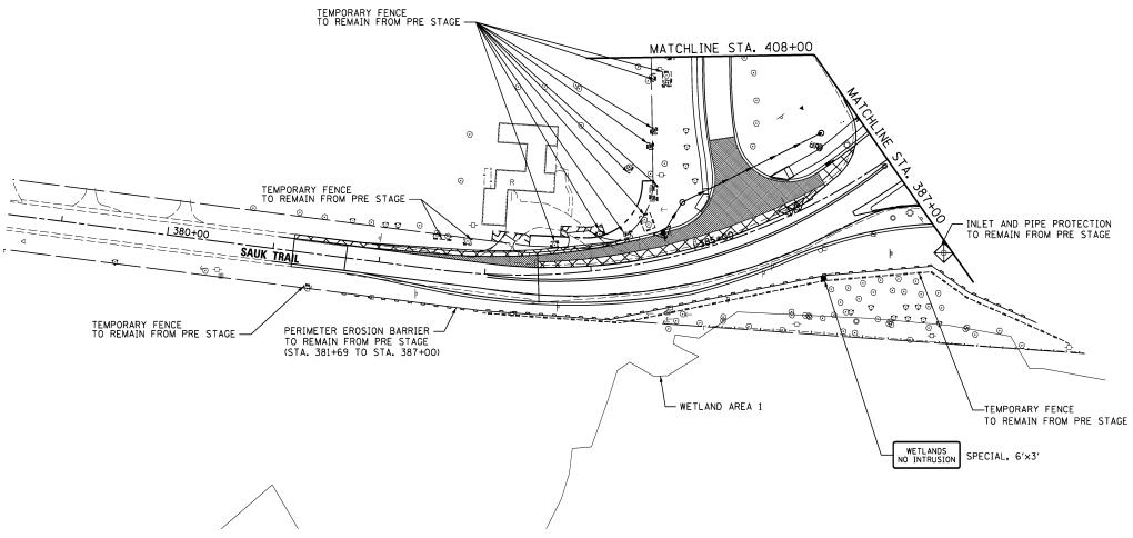
NOTES: INLET FILTERS INSTALLED DURING PRE STAGE SHALL BE MAINTAINED THROUGH REMAINING STAGES UNLESS OTHERWISE DIRECTED BY THE ENGINEER.
