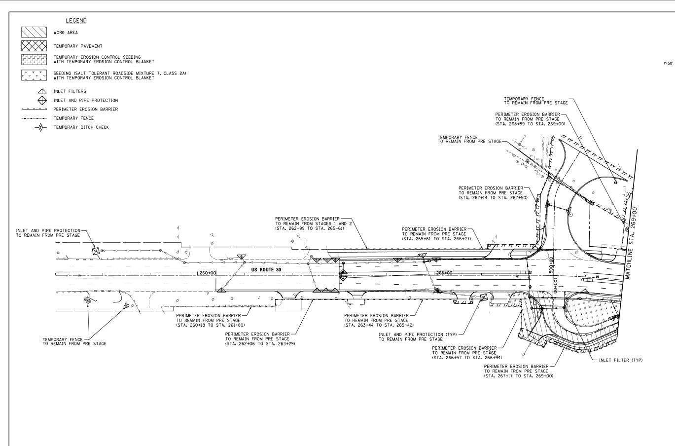
NOTES: INLET FILTERS INSTALLED DURING ALL PREVIOUS STAGES SHALL BE MAINTAINED THROUGH REMAINING STAGES UNLESS OTHERWISE DIRECTED BY THE ENGINEER.
