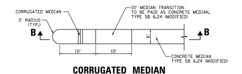
NOTE: CORRUGATED MEDIAN SHALL BE CONSTRUCTED IN ACCORDANCE WITH APPLICABLE PORTIONS OF STANDARD 606306
