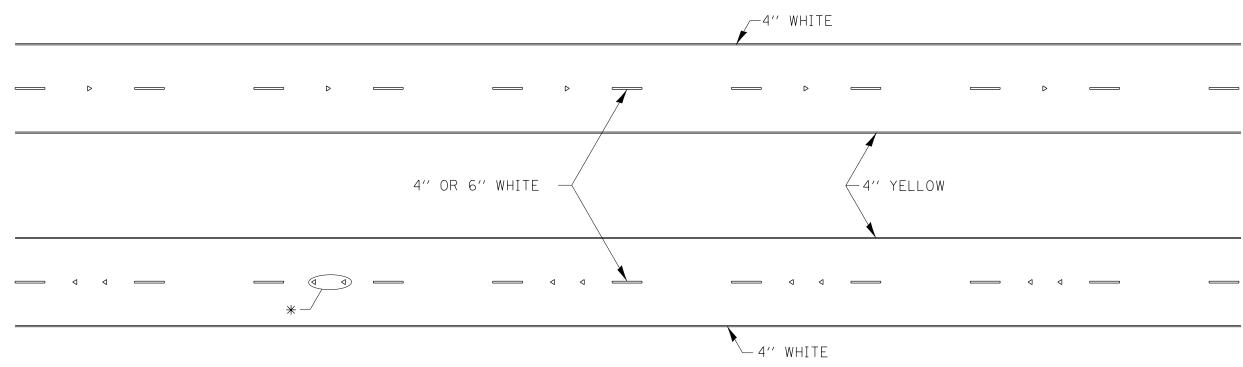
\* SEE HIGHWAY STANDARD 781001 FOR SPACING DETAILS. USE DOUBLE MARKERS WHEN ADT  $\geq$  20,000.
