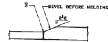
FLANGE @ THICKNESS TRANSITION
