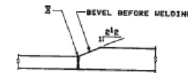
FLANGE @ THICKNESS TRANSITION
