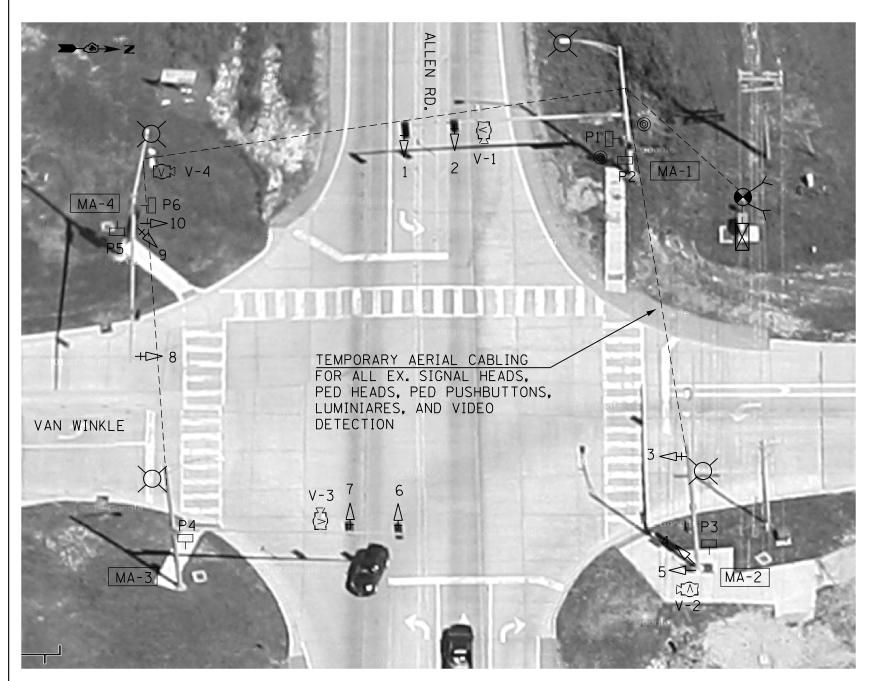
PEDESTRIAM PHASES 2 AND 6 WILL NOT BE UTILIZED IN THE TEMPORARY TRAFFIC SIGNAL INSTALLATION.
