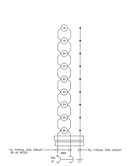
WIRING DIAGRAM (PROPOSED CONTROLLER # 1)
