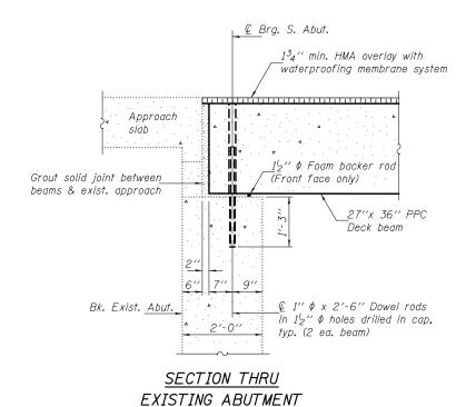
1<sup>l</sup>2" ¢ Foam backer rod Non-shrink grout— (Front face only) Fabric brg. pad (1) 9" x 1" x 12" (interior edges) Dowel rod-⊈ Brg. & dowel rods — Non-shrink grout Bk. Exist. S. Abut. Front face of exist. abut. cap Fabric brg. pad
