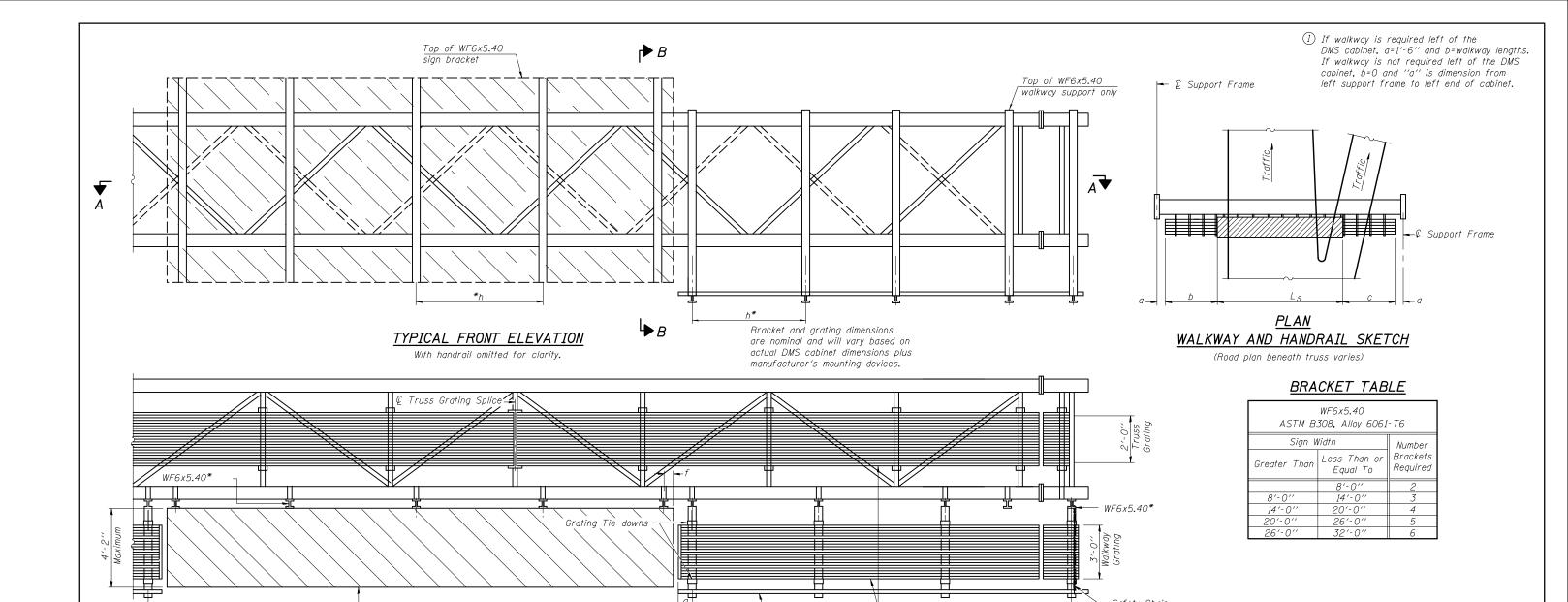
Truss grating to facilitate inspection shall run full length (center to center of support frames) ±12" on overhead trusses.
