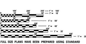
FULL SIZE PLANS HAVE BEEN PREPARED USING STANDARD ENGINEERING SCALES. REDUCED SIZED PLANS WILL NOT CONFORM TO STANDARD SCALES. IN MAKING MEASUREMENTS ON REDUCED PLANS, THE ABOVE SCALES MAY BE USED.
